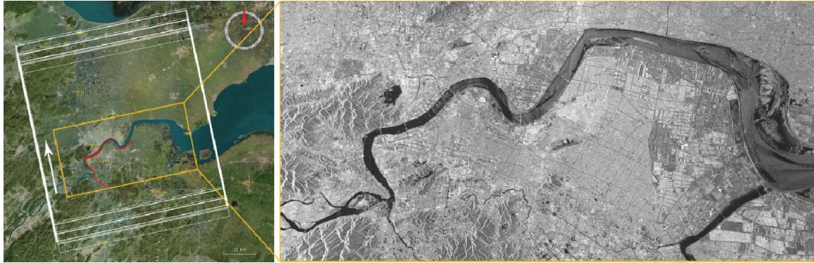
Fig.1 Location of the study area and the SAR amplitude image averaged from 31 ASAR images (Left: The base map is a microsoft bing aerial photo; white rectangles denote the coverage of 31 ASAR images; the white arrow denotes the satellite flight direction; the orange rectangle denotes the coverage of the study area; the red curves denote the leveling routes)
